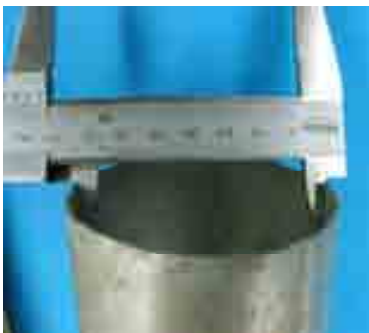
Figure 3.4: Measuring the diameter of cylinders to determine the bulk density of the soil.
