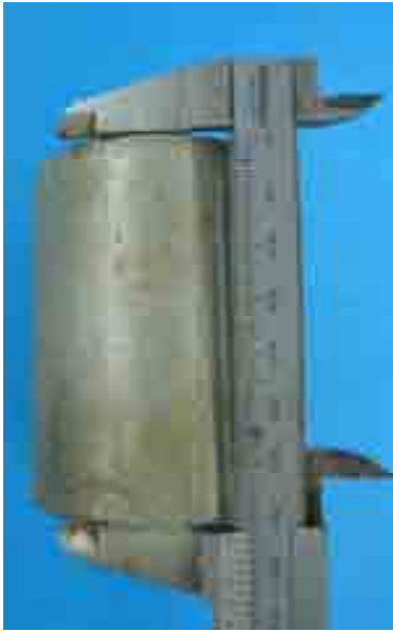
Figure 3.3: Measuring the height of cylinders used to measure the bulk density of the soil.
