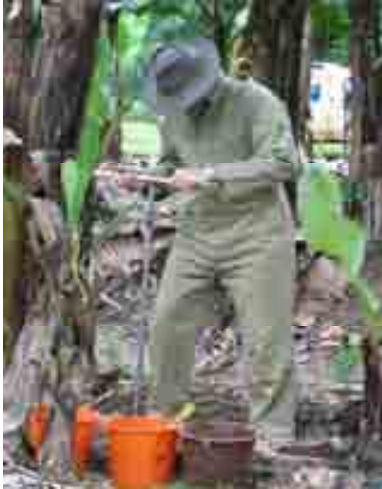
Figure 4.1: Soil cores from banana fields should be taken randomly across the banana paddock and bulked together.
