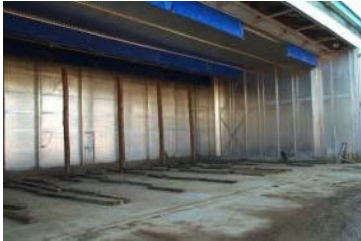
Figure 9.11. Bolster and baffles in a modern batch predryer
