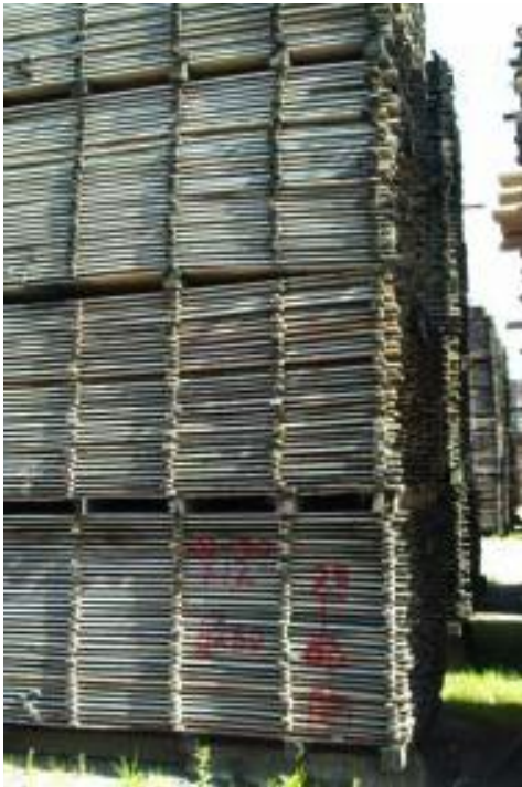
Figure 8.47. Missing bearers cause board distortion
