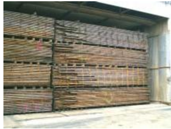
Figure 11.13. Undesirable: Baffling incorrect
