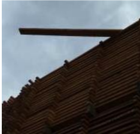
Figure 8.34. A board blown out of position. If this occurs, stack tops should be tied down securely
