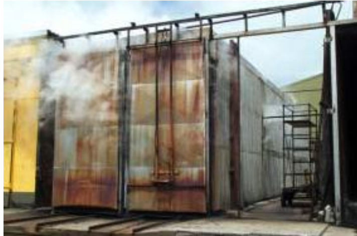
Figure 10.04. Reconditioner in operation
