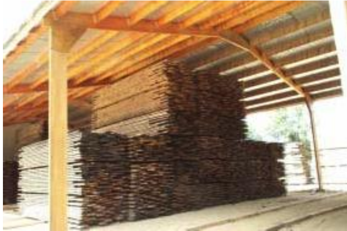
Figure 11.14. Racks positioned under cover
