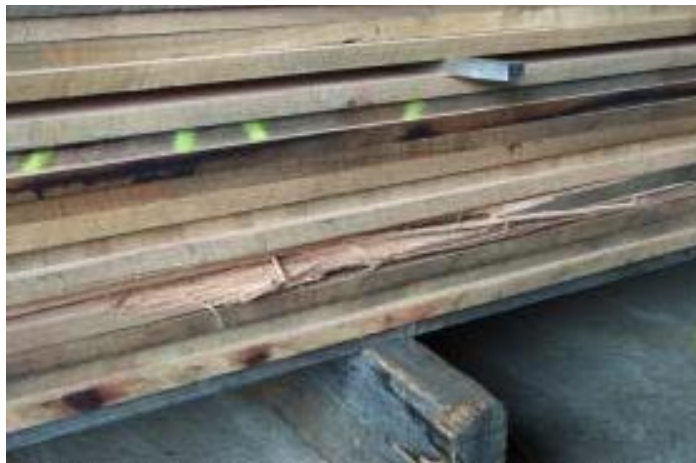
Figure 12.13. Forklift damage to a KD pack
