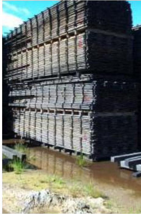
Figure 8.43. Poor drainage leaves stacks standing in water. This slows drying, especially in the bottom rack
