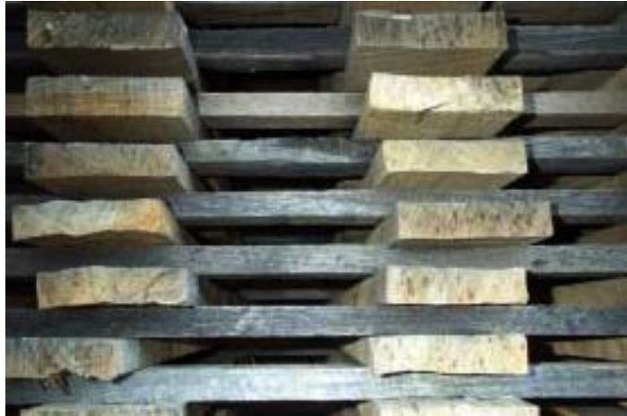
Figure 10.02. Collapse in boards before reconditioning
