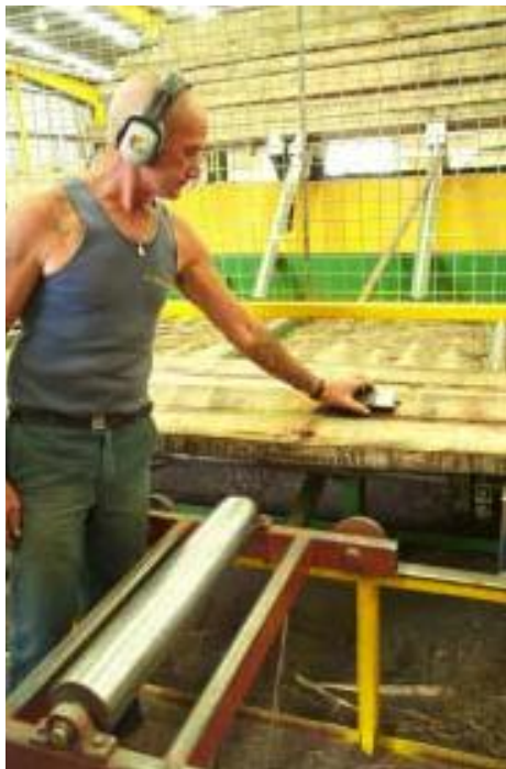
Figure 12.10. Assessing the moisture content of incoming timber with a capacitance moisture meter at a deracker
