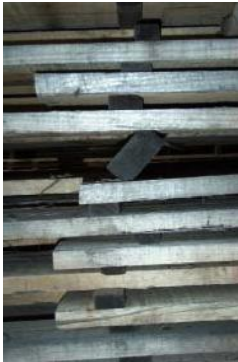
Figure 8.45. Poor handling placement knocks bearers out of line in stacks and causes board distortion
