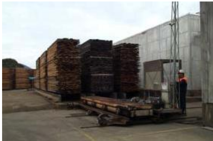
Figure 10.05 Traverser preparing to load a stack for the reconditioner
