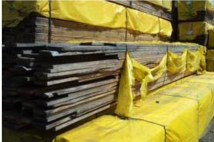
Figure 13.05. Plastic wrapping damaged after prolonged storage outside. The longer material is stored in the open, the greater the chance of significant moisture damage
