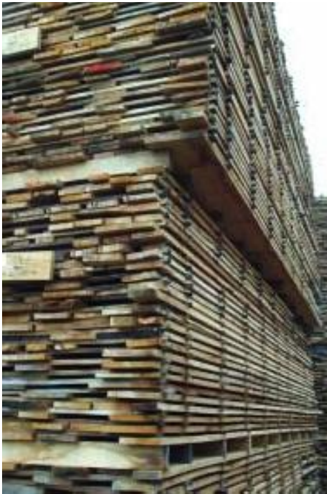
Figure 8.46. Racks out of line in stacks leads to uneven airflow and concentration of load on some boards
