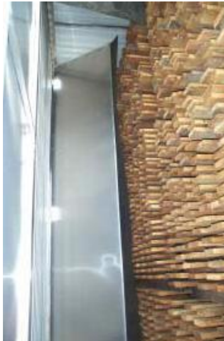
Figure 9.02. A hinged solid baffle with a flexible edge in position in a predryer. Square ended racks are essential for effective baffling
