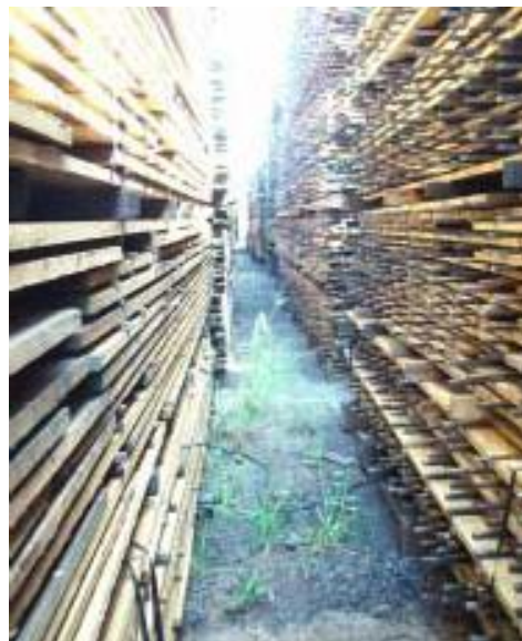
Figure 8.05. The arrangement of racks can modify ambient conditions
