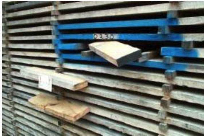
Figure 16.06. Sample board with two outside cover boards
