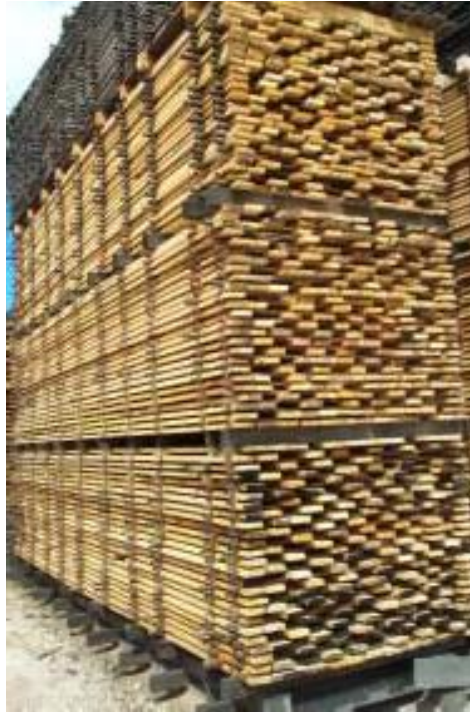
Figure 8.02. A lower value rack on the top of the stack protects the higher value material below
