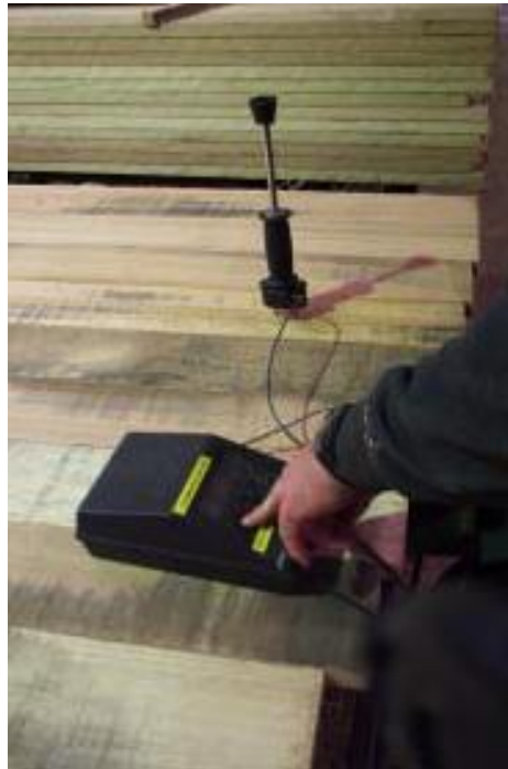
Figure 12.02. Checking moisture with a resistance meter
