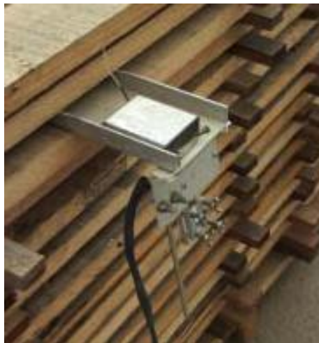
Figure 9.17: An EMC wafer used in a predryer
