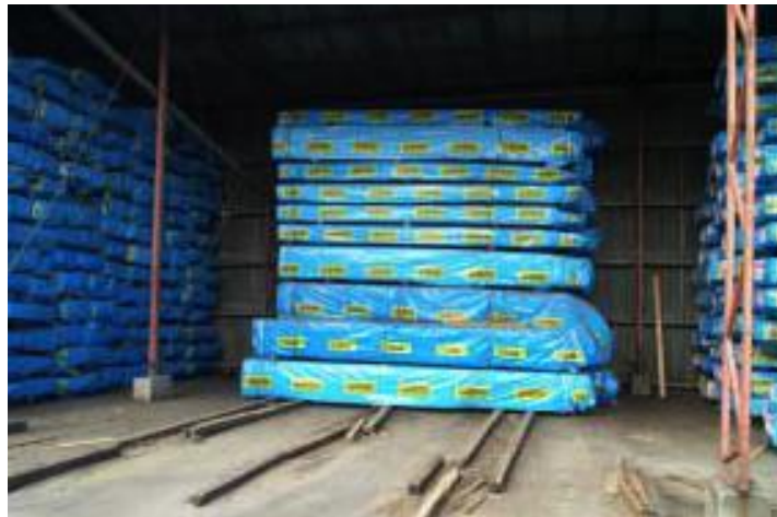
Figure 13.02. Fully wrapped bundles stored in an open sided shed
