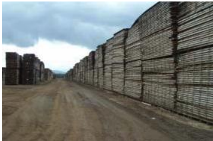
Figure 8.24. Wide main alley in a gravel surfaced drying yard
