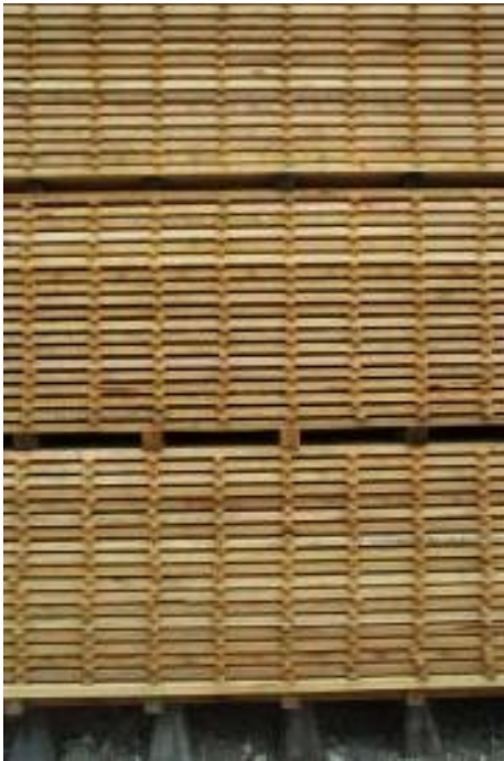
Figure 8.11. A well constructed stack with rack stick, bearers, and piers aligned one over the other
