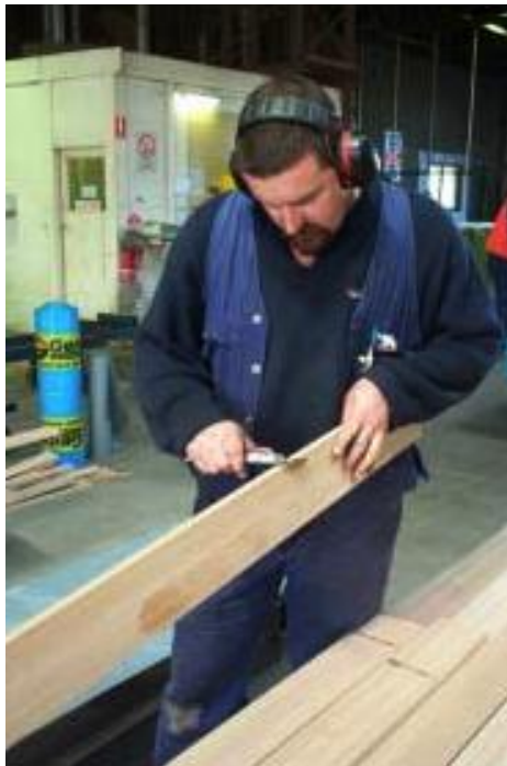
Figure 12.09. Checking the dimensions of a dressed board in the dry mill
