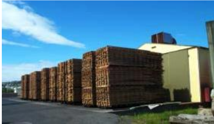
Figure 9.05. Stacks ready to be pushed into the wet end of a series of progressive predryers
