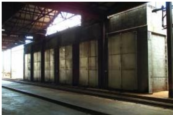
Figure 11.05. A bank of kilns built from masonry
