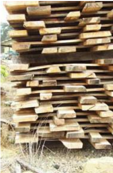
Figure 8.42. Poor rack construction and bearer placement leads to unstable stacks and twisted boards
