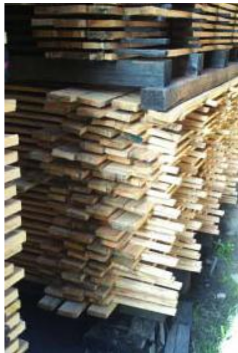
Figure 8.42. Poor rack construction and bearer placement leads to unstable stacks and twisted boards
