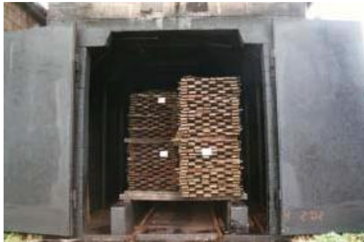
Figure 11.03. Concrete hobs and rails for use with a traverser trolley. Beams spanning between the kerbs should have no noticeable deflection
