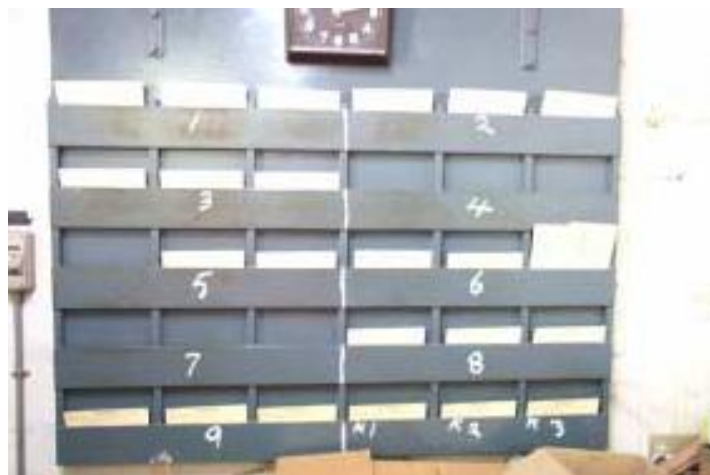
Figure 14.04. Rack cards stored in pigeon holes that correspond with positions in predryers
