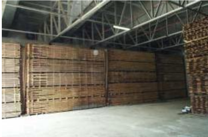
Figure 9.19. Same length racks in a predryer
