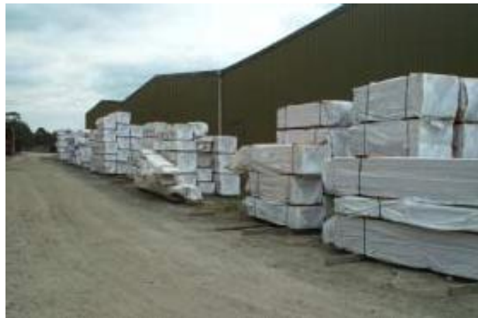
Figure 13.04. Material stored in the weather may be exposed to moisture variation
