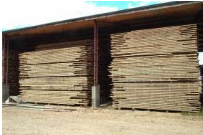
Figure 8.07. Open fronted sheds protect stacks during initial drying
