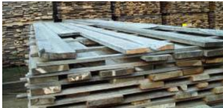
Figure 8. 01. Exposure damage to the top rows of a stack
