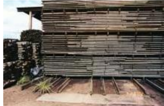
Figure 8.31 Undesirable - Not repeating the position of bearers and gluts under the upper ones
