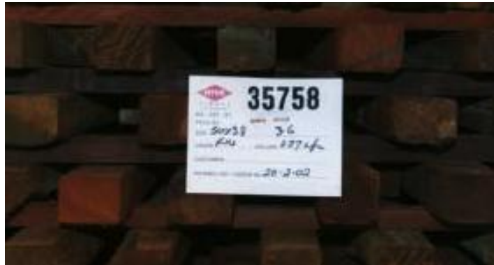
Figure 14.01: Rack tag with its unique identification number and key product information
