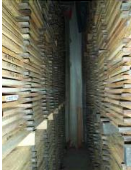
Figure 9.20. Baffles in a progressive predryer
