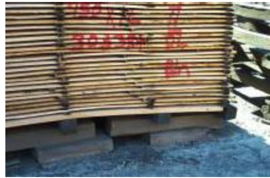
Figure 8.29. Bearer not under the end rack stick line
