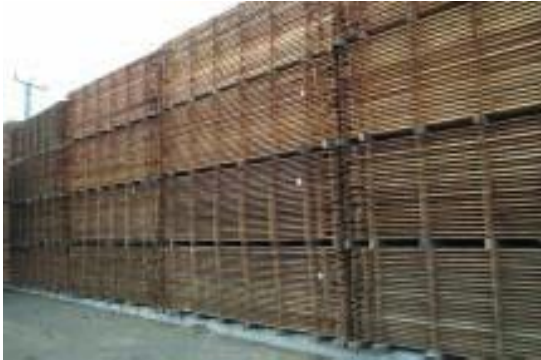
Figure 8.30. Desirable - Repeating the position of bearers and gluts under the upper ones
