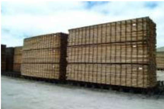
Figure 8.35. Desirable: space under stacks neat and clean
