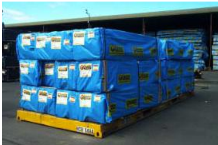
Figure 13.03. Fully wrapped material on a bolster ready for shipment
