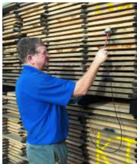
Figure 8.41 Checking the air dry moisture content
