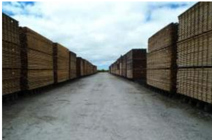
Figure 8.06. A straight and clean drying yard in a cool temperate climate
