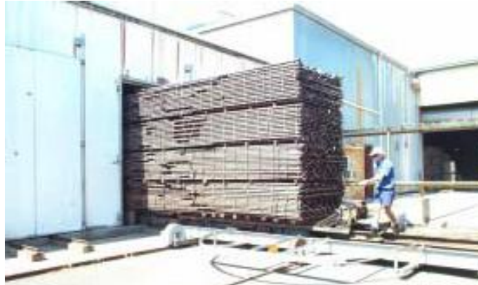
Figure 9.03. A stack of timber being loaded into a large batch predryer on a traverser
