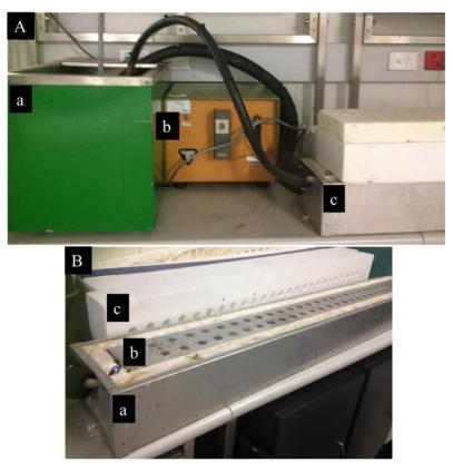
**Fig. 2.6** A: Temperature gradient block set up with associated apparatus; a) chilled water bath unit, b) refrigeration unit, and c) the temperature gradient block. B: a) Temperature gradient block with; b) drilled holes in positions ranging from low temperature (left) to higher temperature (right), and c) insulation. The far end is connected to a heating unit to maintain the higher temperature at desired level.
