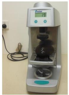
Fig. 2.4 The Sinclair Internal Quality Firmness Tester. A piezoelectric sensor at the tip of the air-blow bellows taps at four points around the horizontal axis of the fruit and the liquid crystal
