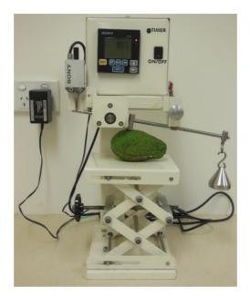
**Fig. 2.5** Anderson<sup>®</sup> Electronic Firmometer. A 9 mm diameter probe contacts the fruit under a load of 200g applied on a lever arm for 10 sec. The objective value of firmness is displayed (mm).
