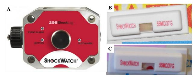
**Fig. 2.9** A: A ShockLog device used to record impact magnitudes and events (<u>http://www.shockwatch.com/products/impact-recorders/shocklog-298/</u>). B: An un-triggered impact indicator clip of 37G attached to an avocado fruit tray. C: An impact indicator clip that has changed colour to red due to an imposed impact event above the threshold limit.
