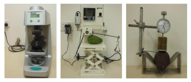
Fig. 1: Avocado cv. Hass fruit firmness measurement with the Sinclair Internal Quality Firmness tester (left), the Electronic Firmometer (centre) and the Analogue Firmness Meter (right).
