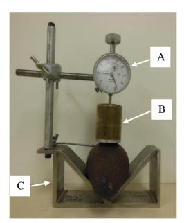
**Fig. 2.1** Analogue firmness meter used for firmness (mm) assessment of avocado cv. 'Hass' fruit. The round dial gauge (A) is manually to zero and then fruit is placed under a 0.5 kg load (B) for 30 sec in a fruit holder (C). Fruit deformation in mm is recorded.
