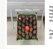
Impact recording device and shock loggers were used in these experiments for their calibration for further use in the supply chain studies.
