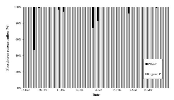
**Figure 11**. Phosphorus speciation as a percentage of the total in the inflow and outflow of the settlement pond at Farm A (Paired columns represent inflow on the left and outflow on the right).
