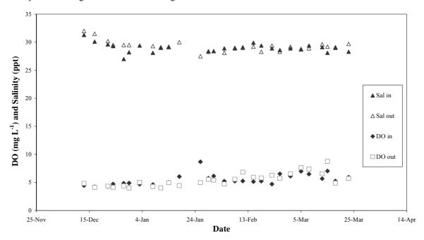
**Figure 2**. Dissolved oxygen concentrations and salinity of water flowing into and out of the settlement pond at Farm A.
