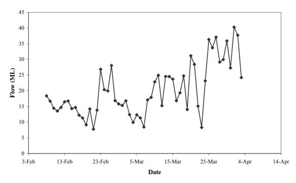
Figure 4. Daily water flow through the settlement pond at Farm A from 8/2/02 to 3/4/02.
