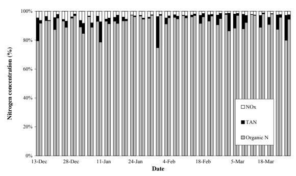
**Figure 6**. Nitrogen speciation as a percentage of the total in the inflow and outflow of the settlement pond at Farm A (Paired columns represent inflow on the left and outflow on the right).
