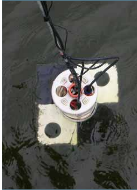
Figure 3.8 (left) The secchi lowered into the water column until it disappears from view
