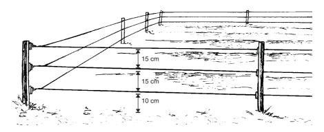
Figure 13. A diagram of an electric fence to exclude hares and rabbits
