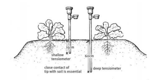
*Figure 15.* A monitoring site illustrating placement of the shallow and deep tensiometers.
