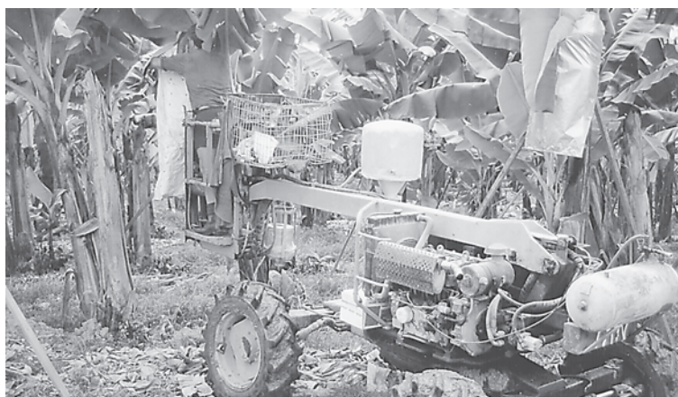
Figure 23. Bagging and spraying bunches from a 4WD bagging machine
