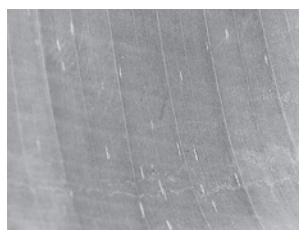
Stage 2a (early streak) Specks become 3 – 4 mm x 1 mm long streaks, increase in length and turn yellowish.
