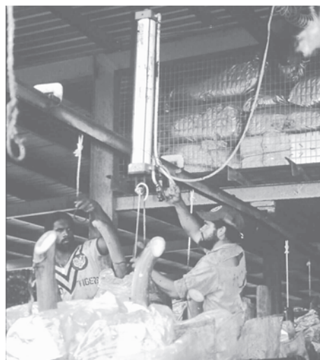
Figure 25. Hanging bunches on a bunchline using a pneumatic bunch lifter
