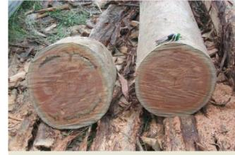
**Figure 3.3** Butting the log to remove defect associated with the stump, which in this case was most likely an old fire scar.
