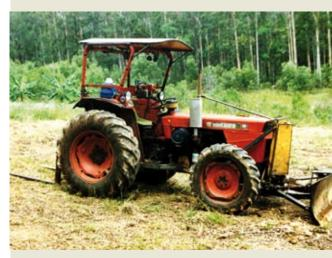
**Figure 1.3** The tractor used for the harvest was a 60 hp 4WD with blade and rear forks.
